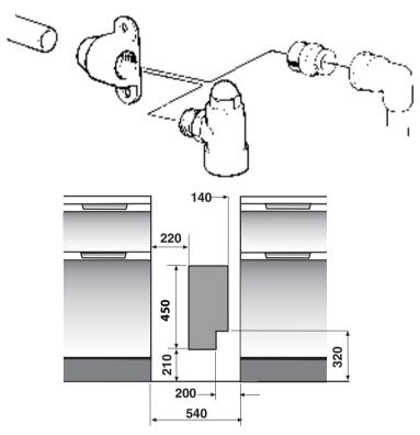
Connection to the cooker should be made with an approved appliance flexible connection to BS 669. A length of 0.9 to 1.25m is recommended. The length of hose chosen should be such that when the cooker is in situ, the hose does not touch the floor.
